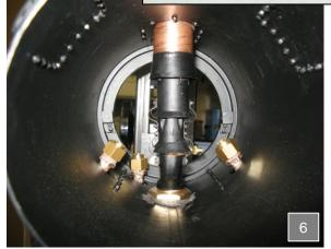
So, when the parallel chimney part is slid down from the top of the chimney onto the sliding joint the whole assembly becomes rigid. **(photo 6)**
