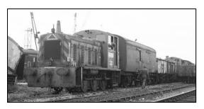
An 0-6-0 diesel shunter was used to extricate the vehicle from the train of assorted wagons destined for scrap
