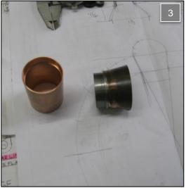
a gentle bit of pushing and shoving at the right places is necessary to get the whole thing concentrically bent for silver soldering.
